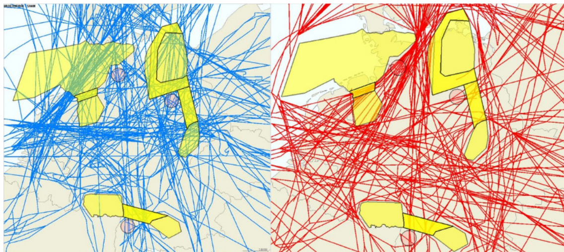
Figure 16: Flight Tracks without (blue) and with (red) Re-Routing Measures
