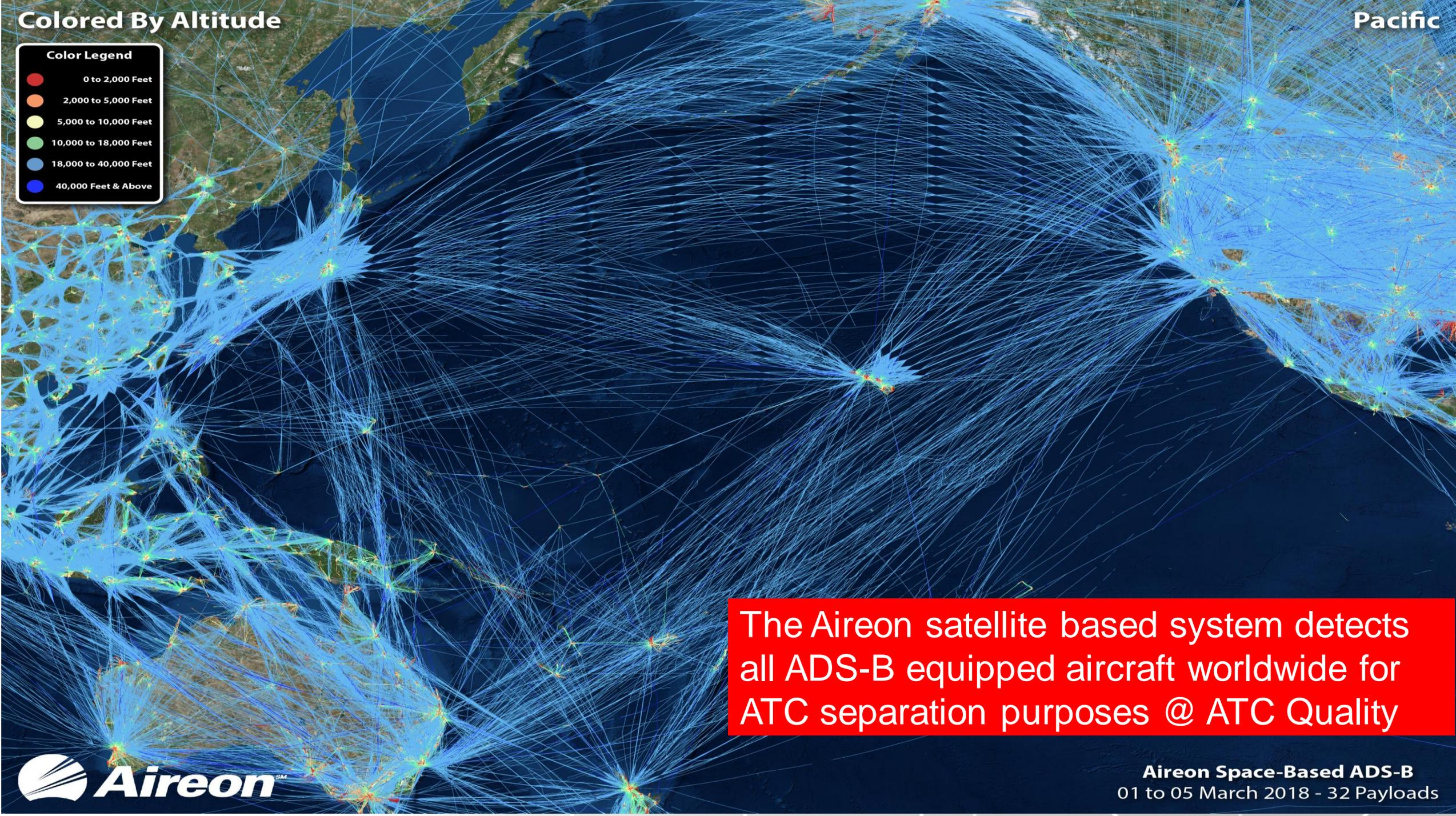
The Aireon satellite based system detects all ADS-B equipped aircraft worldwide for ATC separation purposes @ ATC Quality
