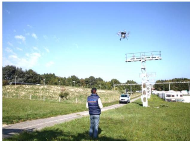
The installation of SIS inspection systems in RPAS allows expanding the scope and possibilities of ground measurements, providing benefits both to the Air Navigation Service Provider, as well as to the Aeronautical Authority in the certification and extension of certification periods for radio navigation aids, including:
