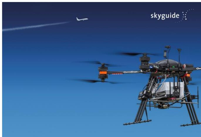
Skyguide, the provider of air navigation services in Switzerland, is a leader in the development and use of mobile inspection systems for the maintenance, setup and certification of radio navigation aids, capitalizing under this figure of payload in a RPAS, systems that they have been developing and using for more than 10 years for the measurement of radio navigation aid signals in the field.
